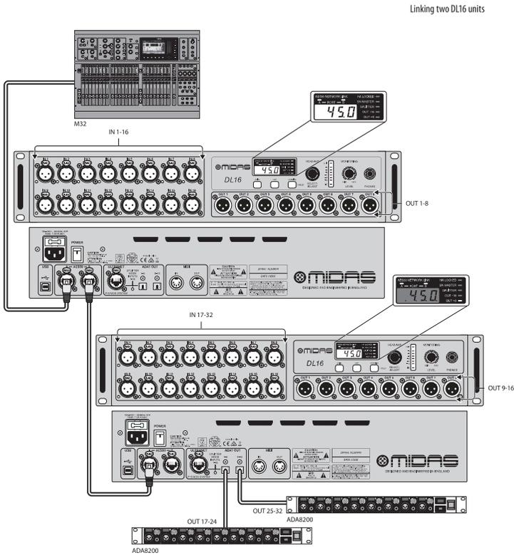
**Note:** The signals on both DL16 units (Out 1-8 and 9-16) and both ADAR200 units (Out 17-24 and 25-32) are fully defined on the M32's 'Routing/AESSO Output' page. The second DL16's outputs must be set to Out +8 on the unit itself.
