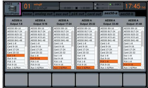
The following chart details the signal flow to and from the stage when using 3 DL16 units.
