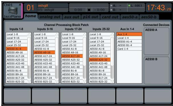
Signals sent from the M32 to the stage are seen the same on all DL16 units in the chain. AES50 channels 1-8 will appear on the XLR OUTPUTS of each unit. To achieve maximum output to the stage, the 2nd and 3rd units in the chain must have their physical OUTPUTS set to OUT +8 and OUT +16 respectively.
