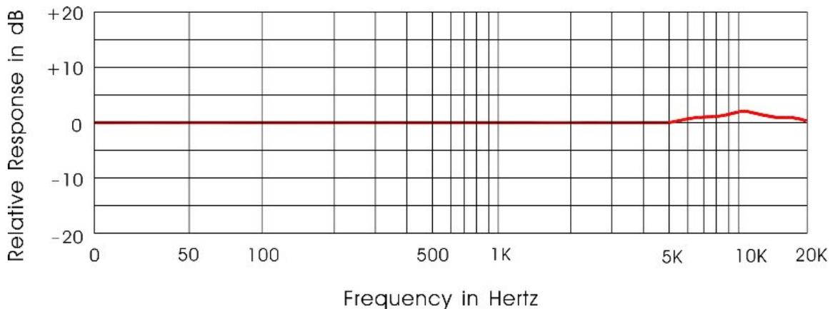
The RTA-M is an omni-directional, flat frequency measurement microphone specially designed for the Driverack series to pick up all frequencies from 20 Hz to 20 kHz , ensuring accurate "pinking"/real-time analysis of your audio. It runs on phantom power (supplied by the Driverack units) and comes with a clip and case.
