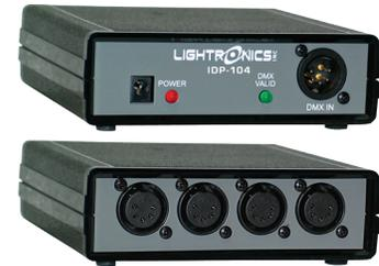
The IDP104 is an optically isolated DMX splitter with one DMX input and four independent DMX output circuits.
