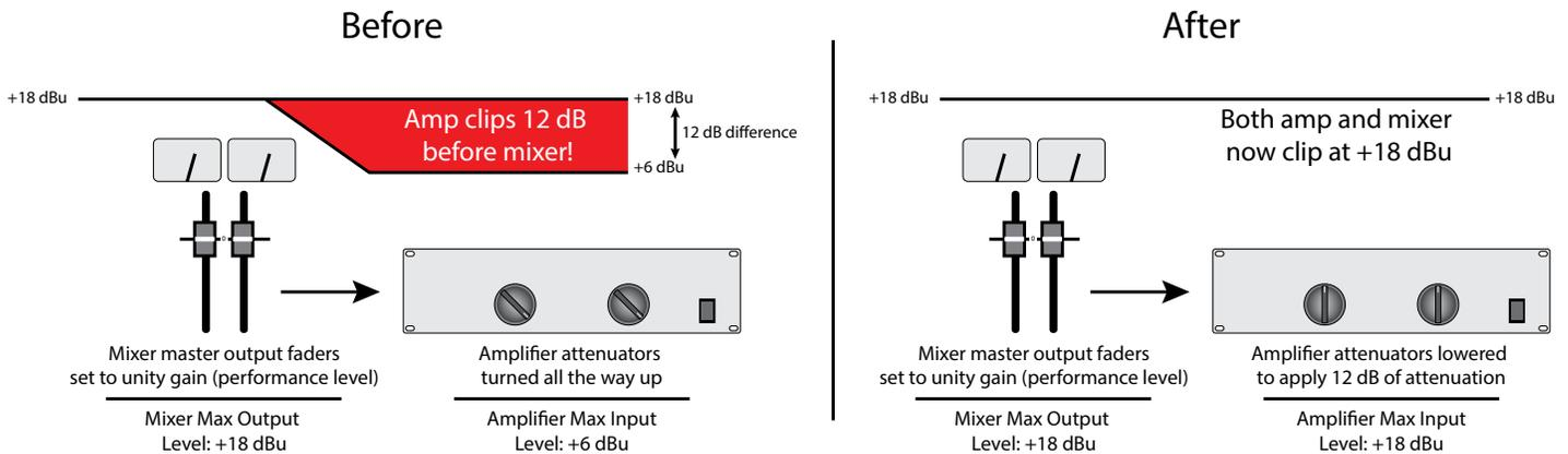
One way to set up your gain structure is to play pink noise through the entire system and adjust each gain stage in the signal chain in succession using the clip indicators on each device. If there is no clip indicator on your mixer then use the output meters; most reputable console manufacturers use red LEDs at the top of the meters to show the onset of clipping.
