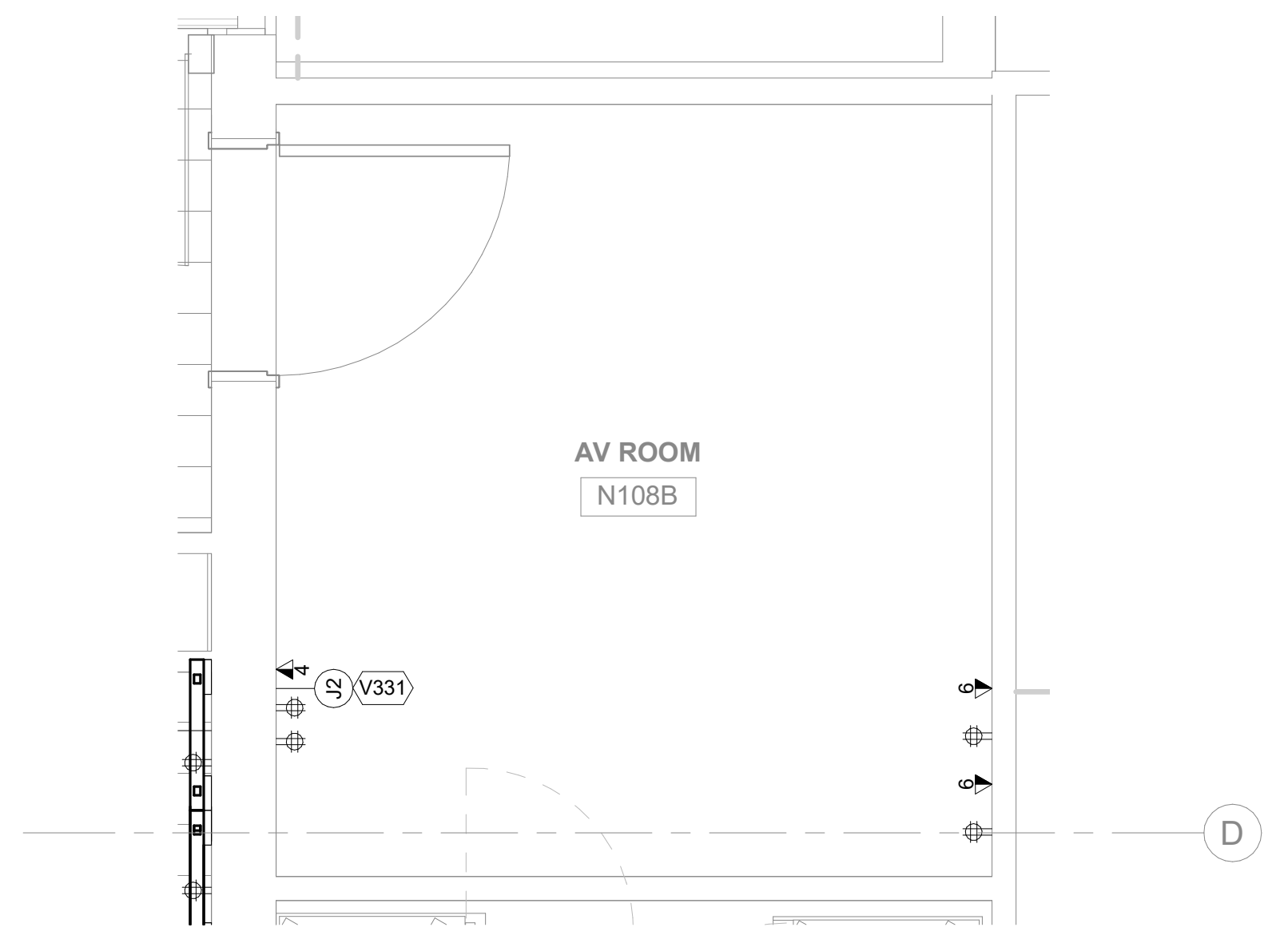
3 AUDIOVISUAL ENLARGED ELECTRICAL PLAN - ROOM N108B 1/2" = 1'-0"
