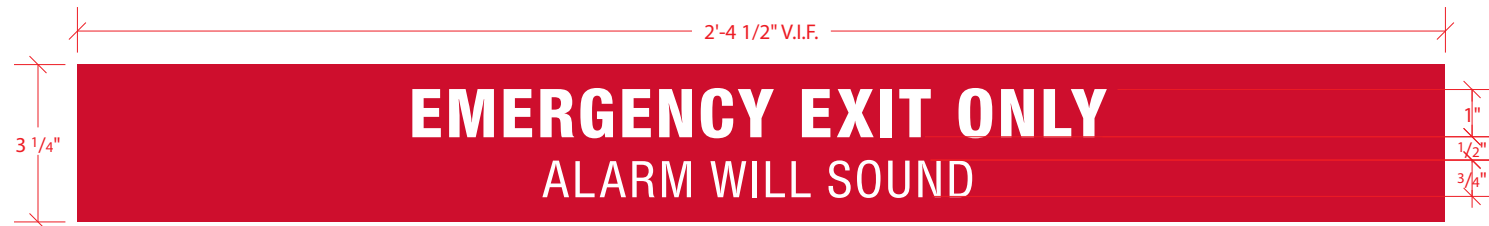
S8 EMERGENCY EXIT DOOR BAND
