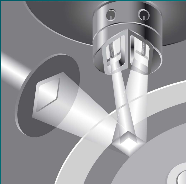
Variofocus creates a number of tailored focal spot sizes
