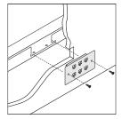
NEMA-size communication outlets (single gang) do not require a Steelcase faceplate. Cannot be used in base.
