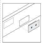
Communication outlets attach to openings in panel base trim. Order communication outlets from an outside vendor. Knockouts for communication in base accommodate modular furniture size only.
