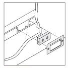
Faceplate is used to surround modular furniture size communication or DECORA outlets when installed in the face of a tackable acoustical panel skin. Templates for field cutting are available through Service Parts (T500940SR).
