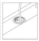
Feed-through horizontal connecting bar cable sleeves can be added in the field to finish the exposed metal edges of vertical cable passthrough openings.
