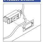
Faceplate, ordered separately, is used to surround receptacle when skin is field-cut. Templates for field cutting are available through Service Parts (T500940SR).
