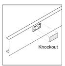
Knockouts in base trim can be removed in the field where needed. Knockout dimensions are 13/8"H by 25/8"W.
