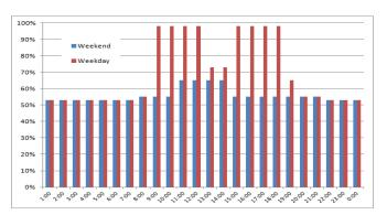
\*Fume Hood Diversity Schedule is the standard taken from ASHRAE 90.1-2007 App. G. Energy usage and cost are calculated using values which maintain the minimum safe nozzle velocity for the specified fans.
